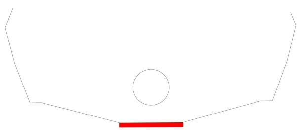
Rear Typical view showing wear plate on delta in RED
