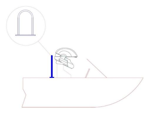
Side sketch of typical craft showing BLUE head protection loop fitted. Note top of loop is as close to centre of helmet for occupant as possible.
